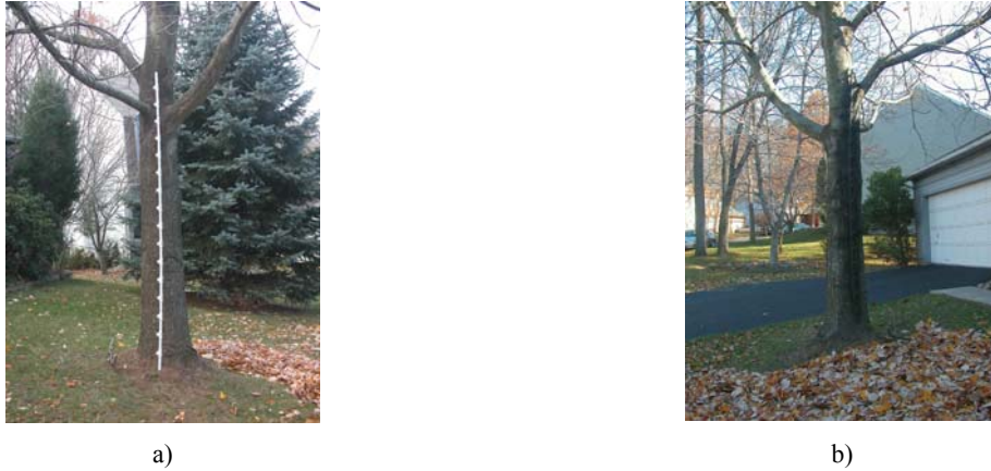
Fig. 5. Example camouflage of sparse detector sensor: a) Profiling sensor realized with sensing elements in PVC pipe and mounted on a tree b) Profiling sensor realized with sensing elements in PVC pipe painted to blend in with a tree.
