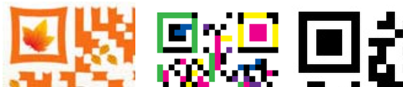
Figure 3. Partial view of Symbols 1 and 10, showing the position detection pattern damage and what the pattern should look like on the right.
