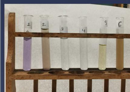
**Figure 3.** Same set up as figure 1, except with the activated carbon instead of the magnetite-activated carbon. Only difference is test tube 2, which contains the water that the Activated Carbon alone decontaminated.
