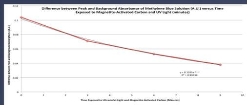
**Figure 8.** The graph of the dissociation of Methylene Blue with  $2\text{Fe}_3\text{O}_4$ +Activated Carbon. The absorbance decreases in an exponential fashion, and the exponent is -0.321.
