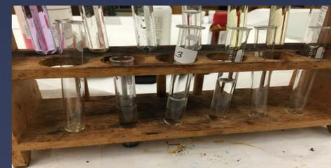
**Figure 4.** Same set up as figure 1, except with two times the  $\text{Fe}_3\text{O}_4$  and activated carbon inside. The only difference is test tube 2, which contains the water which the powder containing twice the magnetite decontaminated.
