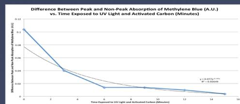
**Figure 7.** The graph showing the dissociation of Methylene Blue with Magnetite-Activated Carbon. The absorbance decreases almost in a linear fashion, and the slope is equal to -0.11.
