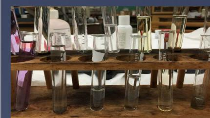
**Figure 2.** The final appearance of the experiment. Test Tube 1 contains 5 mL of "polluted" water with 0.1 M Sodium Hydroxide. 2 contains 5 mL of the cleaned water, as well as one drop of both 0.1 M HCl and 0.1 M NaOH. 3 contains HCl. 4 Contains NaOH. 5 contains 2 mL of Polluted Water, 2 mL of  $\text{H}_2\text{O}$ . 6 contains the ethanol solution.
