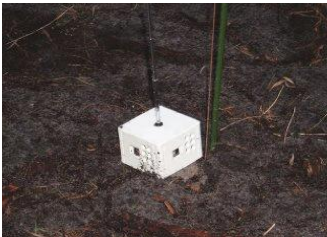
Figure 2: An XSM (Extreme Scale Mote) deployed on the ground in its usual enclosure during the ExScal demonstration.
