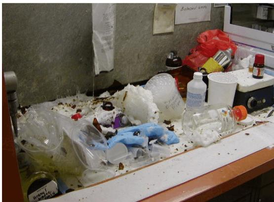
This accident had a happy ending due to two factors: Because it happened at night, no one was around to be injured; because the fume hood sash was lowered prior to leaving the lab, most of the glass and contamination was confined. Were it not for the timing and lowered sash, someone could have received a life-threatening injury, and the lab might have been contaminated.
