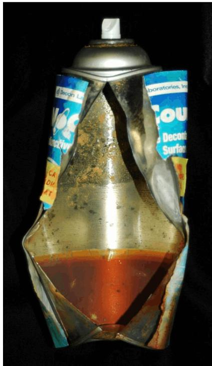
The ruptured can of radioisotope decon spray. Note apparent corrosion inside.
