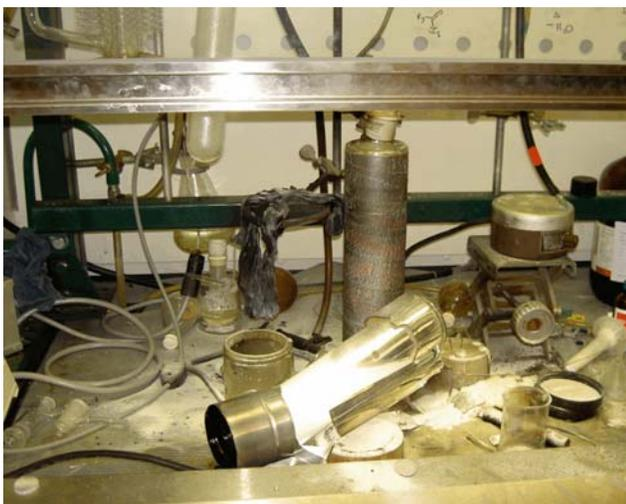
Remains of the laboratory fire include a broken Dewar
