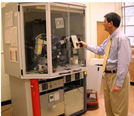
X-ray diffraction unit is surveyed for radiation leakage during annual inspection by EH&S.
