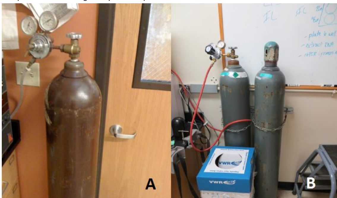
Figure 61: Compressed gas cylinder storage. A-Unsecured cylinder. An unsecured compressed gas cylinder can be very dangerous, particularly if it does not have the cap on it as pictured. The valve can be knocked off if the cylinder were to fall over making the cylinder a very heavy projectile because of the pressure within being suddenly released. B-Secured cylinder. These cylinders are appropriately secured to the wall by a chain and the cylinder that is not in use has the protective cap in place.
