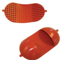
Figure 26: Hot Hands. Hot hands are used for handling somewhat hot objects that have been heated on hot plates. They must not be used for removing items from the autoclave.
