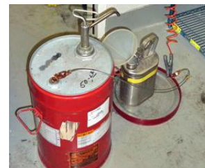
Figure 51: Appropriately Grounded and Bonded Containers.
