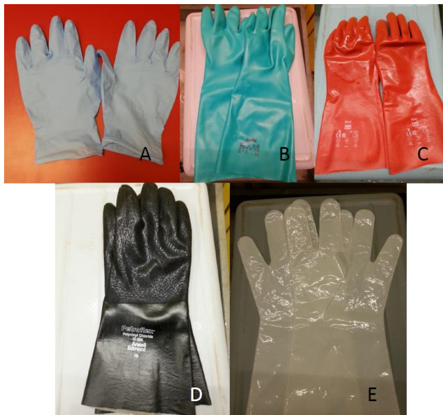
Figure 29: Gloves for chemical hazards. A-Standard nitrile gloves. These are the most common laboratory gloves and they are suitable for use with most chemicals. They are unsuitable for use with halogenated solvents, acetone, phenol or benzene. For complete compatibility discussion, see manufacturer's chemical resistance guide. B-Solvex gloves. These gloves are made of the same material as nitrile; they are just thicker and longer. This thickness reduces dexterity but increases protection. C-Polyvinyl alcohol (PVA) gloves. PVA gloves should be used when large amounts of halogenated solvents (like chloroform) are going to be used. These gloves have limited dexterity and are expensive (~$30 per pair). D-Polyvinyl chloride (PVC) gloves. PVC gloves tend to be more susceptible to chemical breakthrough than nitrile, but there are a few chemicals for which they are more protective than nitrile (like phenol). E-Laminate film gloves. These gloves are resistant to almost every chemical; however, they have very limited dexterity. They should be used as a last resort in a laboratory setting but are good for use in chemical spill cleanup kits.
