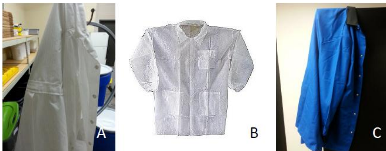
Figure 30: Different types of lab coats. The most common type of lab coats found in the lab is standard cotton lab coats. Here are some examples of alternatives to those coats. A-Fluid-resistant lab coat. This coat does not absorb liquids; it repels them. It is suitable for working with liquid chemicals and is easy to disinfect. B-Disposable lab coat. This lab coat is meant for short-term use and may be suitable for a teaching lab. Once it is gets contaminated, it must be disposed. C-Fire-resistant lab coat. This type of coat must be used when working with materials that may spontaneously ignite. It is made from a fire-resistant material called Nomex.
