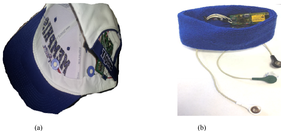
Figure 9. (a) First prototype of the ambulatory EEG NeuroMonitor device inside a cap. (b) Second prototype NeuroMonitor device with smaller footprint can be concealed within a child-sized headband.
