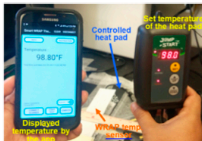
Figure 15. Experimental functional verification of WRAP temperature sensor.
