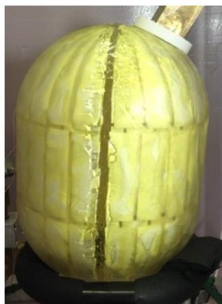
Fig. 1: Completed polymer/aerogel compound tank for NASA grant.
