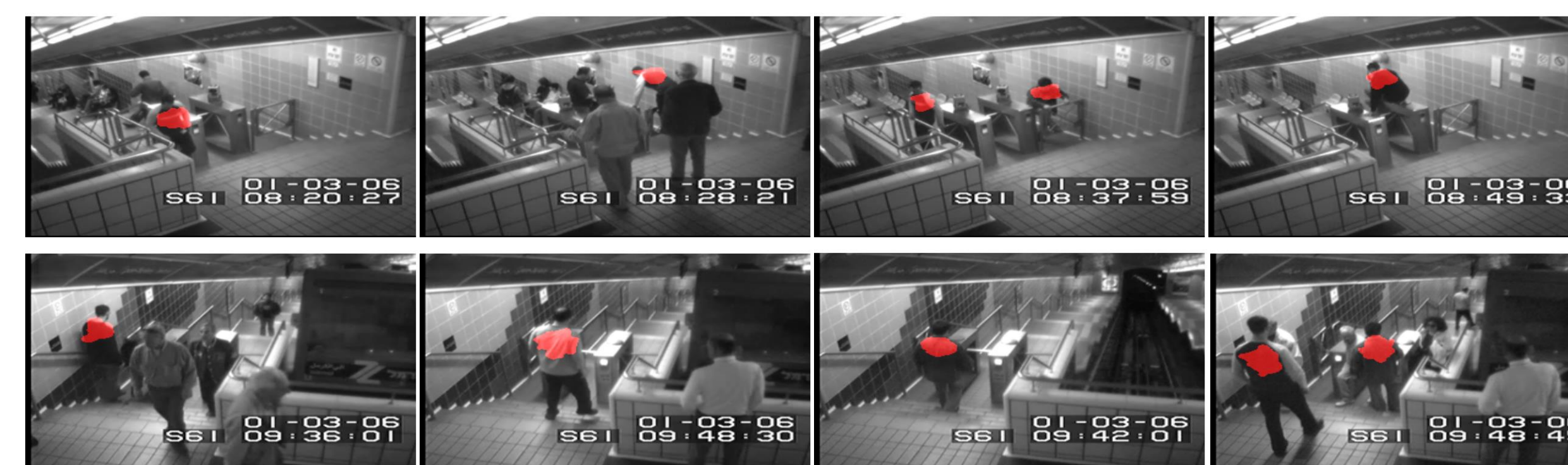
Figure 4: Anomaly detection in Subway dataset. Top row represents entrance gate and bottom row represents exit gate. Anomaly detection includes detection of wrong direction events and no payment events. Anomalies detected by our model are highlighted in red (best viewed in color).
