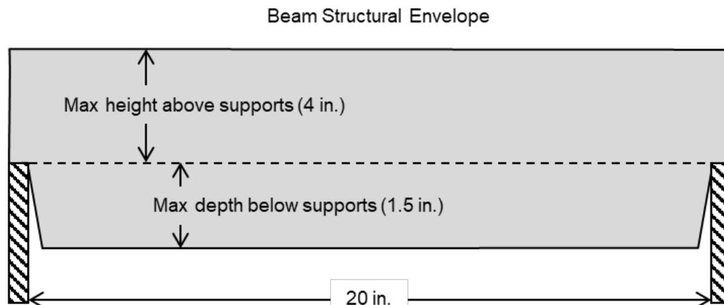
Figure 2. Bridge Supports and Geometrical Constraints
