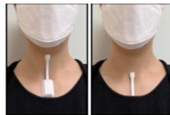
Figure 2: A respiratory acoustic sensor using thin-film electrode technology [2]
