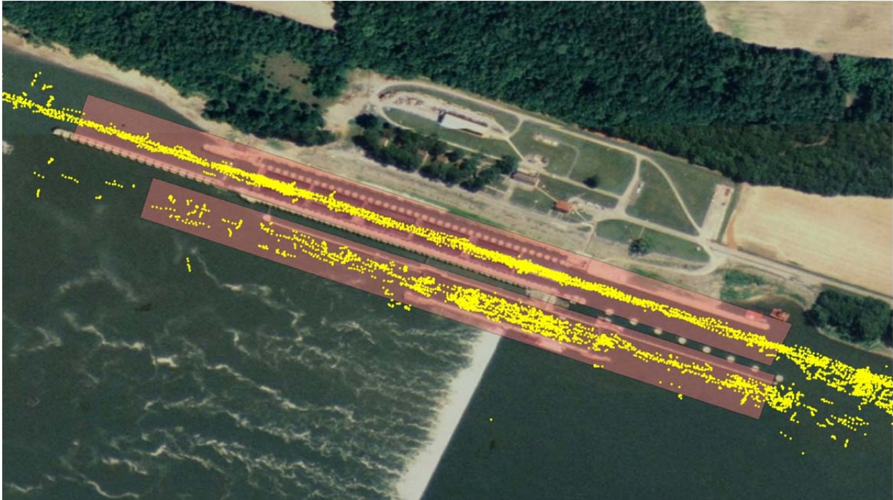
1 2 FIGURE 5 AIS position data at Lock and Dam 52. 3
