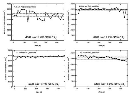
technique to disperse dry powders at a constant rate. The main challenge in doing so is that powders love to stick to surfaces due to their high adhesion energy and are difficult to aerosolize. We have developed a technique that is currently prepared for patenting to generated aerosols from dry powders at high concentrations for AM over long periods of time (see figure).
