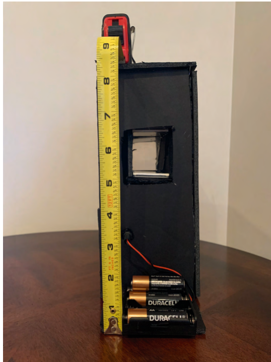
Figure 4. Experimental prototype of the Pepper Ghost Tunnel using cardboard to enclose the transparency film and the two opposed LCDs. The total size of the prototype is 101.6 \times 241.3 \times 190.5 mm (Width \times Height \times Depth).
