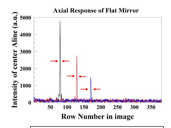
Measured axial resolution of  $1.8 \pm 0.4 \mu m$
