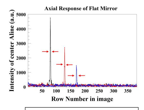
Measured axial resolution of  $1.8 \pm 0.4 \mu m$
